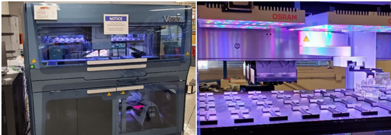
Fig 4: EcoBOT TEAMS — left photo shows the EcoBOT system, right photo shows how the EcoFABs can be arrayed within the EcoBOT.
